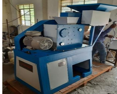
Concrete Laboratory- Jaw Crusher (SRIC)
