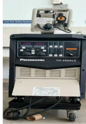
Gas metal arc welding (GMAW)
