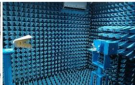
Anechoic chamber Make: Entuple Technologies. Size of Chamber: 3 x 3 x 2.4 m (LWH)
