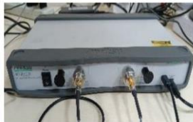
Two Port Vector Network Analyzer (VNA) Make: Anritsu Model: MS46122B
