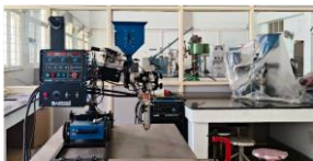
Sub merged arc welding (SAW)
