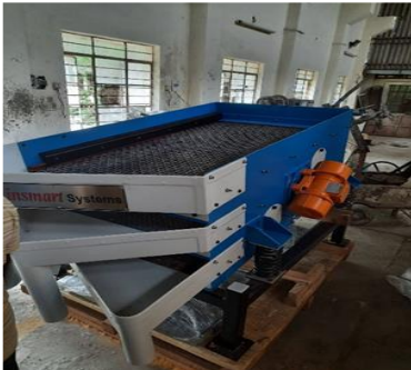
Concrete Laboratory-Segregator (SRIC)
