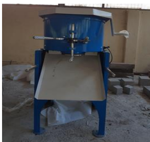
Concrete Mixer (DST)
